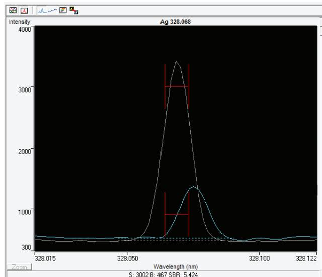
**Figure 1.** Zirconium interference shown to the right of the silver line at 329.068 nm
