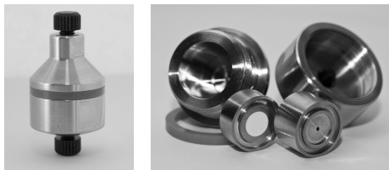
Agilent Bio-Monolith column (left), Bio-Monolith column housing, and monolith disc (right).
